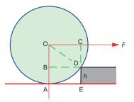
**1.42** Taking torque about D, the corner of the obstacle, (F)CD = (W)BD (Fig. 1.23)
